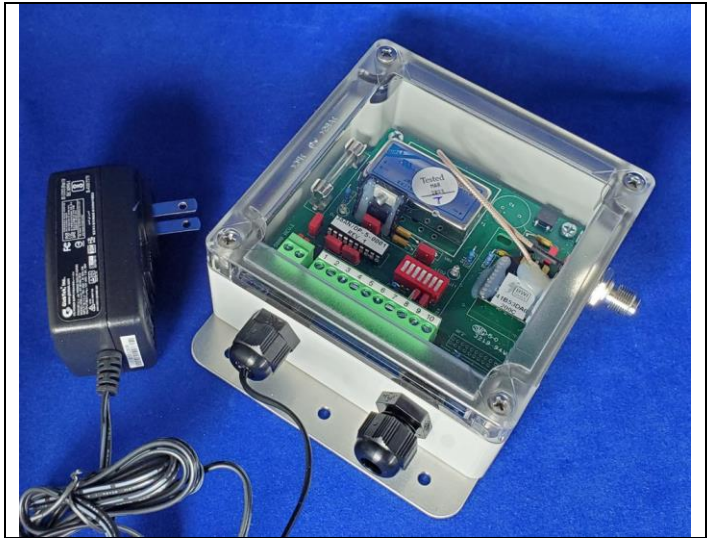
Dimensions (with mounting plate) 6.3" L x 4.8" W x 2.3" H
