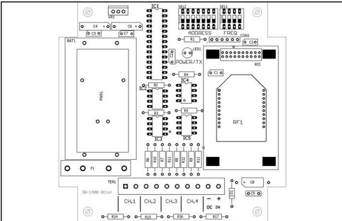
Wire as shown based on number of contact inputs
