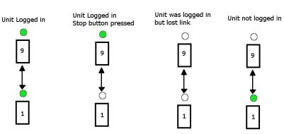
Each remote unit uses a pair of relays to show its state.
