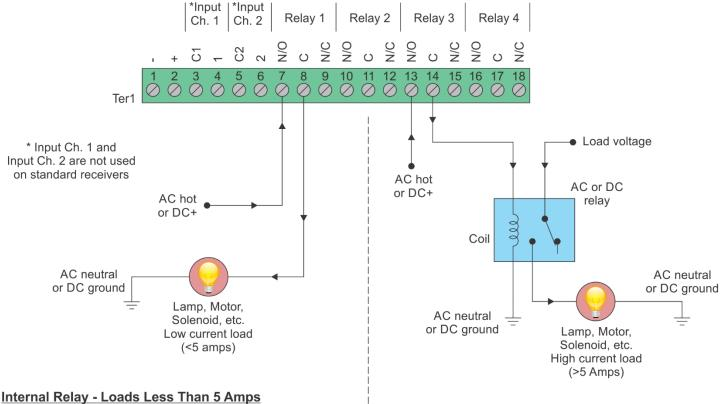
Loads up to 5 Amps may be wired directly to the internal relays. Wiring to the N/O contact will cause the load to turn on when the relay is energized (the load is on when the relay is on). Wiring to the N/C contact will cause the load to turn on when the relay is deenergized (the load is on when the relay is off). AC or DC voltages can be switched through the relay.
