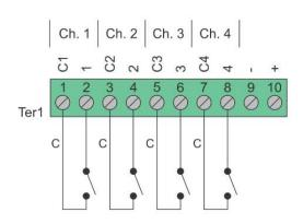
Standard Wiring for Common Ground Applications
